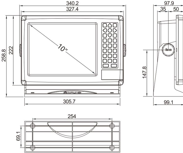
Flush Mounting [Unit:mm]
