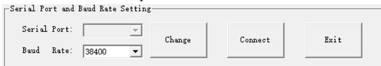
Serial port: Select the serial port which connect to the DB9.
